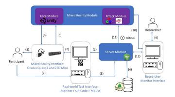
Figure 2: Diagram of our experimental harness.
