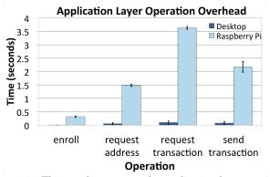
Figure 6: This graph compares the application layer runtime (i.e., excluding communication overhead) of our Braavos prototype running on a desktop and a Raspberry Pi. The latter is lower-end hardware more representative of a possible dongle; even unoptimized, the incurred overhead is acceptable.
