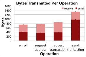
Figure 7: The size of each protocol message in our prototype. We discuss the time needed to send these messages in the text.
