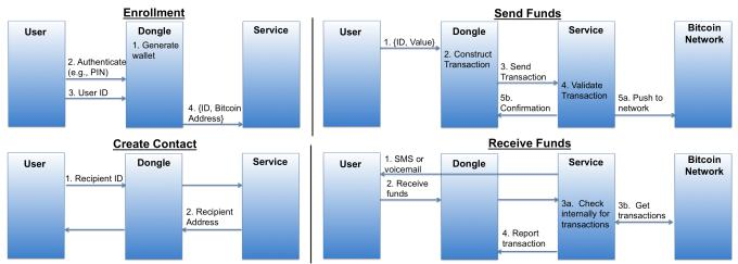
Figure 3: Overview of the Braavos protocols. Note that communications between the dongle and the service are mediated by mobile phones, which have been omitted from the diagrams. Each operation begins with the user authenticating, e.g., via a PIN or fingerprint scan, and communications are encrypted with OTR.
