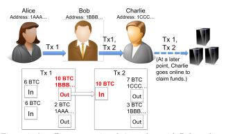
Figure 4: An offline transaction chain, ending with Bob sending Charlie 7 bitcoins. (We use "Tx" as shorthand for "transaction".) Note that (in Bitcoin terms) the input of Transaction 2 corresponds to a particular output of Transaction 1—thus, for Transaction 2 to be considered valid by the service and by the Bitcoin network, both must know about Transaction 1. Hence, Charlie must upload the entire transaction chain to claim his funds.
