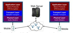
Figure 5: Our modular Braavos prototype implementation, similar to the TCP/IP protocol stack.
