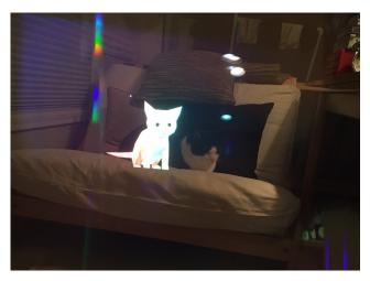
Fig. 2: **Real-World Occlusion.** This photo was taken by a smartphone camera through a HoloLens display (resulting in some reflective camera artifacts). It shows that virtual content displayed by HoloLens (here, a cat) can visually obscure real-world objects (also a cat).
